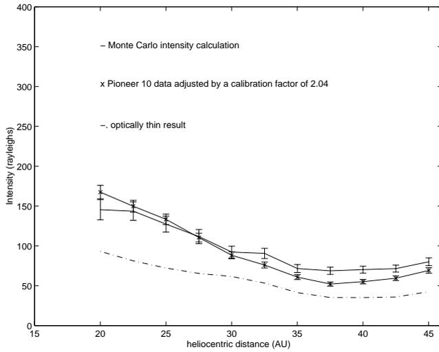
**Figure 4.** Comparison of Monte Carlo optically thick and optically thin calculations using heliospheric model with neutral hydrogen density of  $0.15 \text{ cm}^{-3}$  and proton density of  $0.07 \text{ cm}^{-3}$  and Pioneer 10 Lyman Alpha glow data adjusted by the constant calibration factor as function of heliocentric distance.
