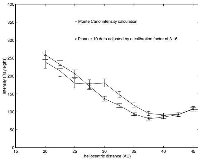
**Figure 5.** Same as figure 4 except that a heliospheric model with neutral hydrogen density of  $0.2 \text{ cm}^{-3}$  and proton density of  $0.05 \text{ cm}^{-3}$  was used
